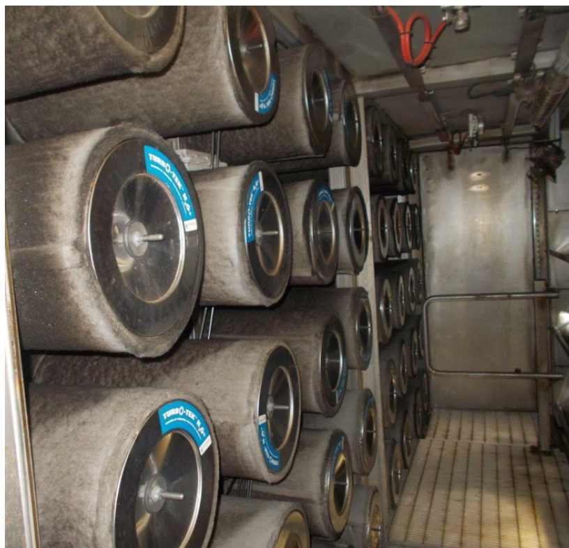
Despite bushfire soot build-up at 6,000 hours, there was little to no spike in differential pressure or blade health.
