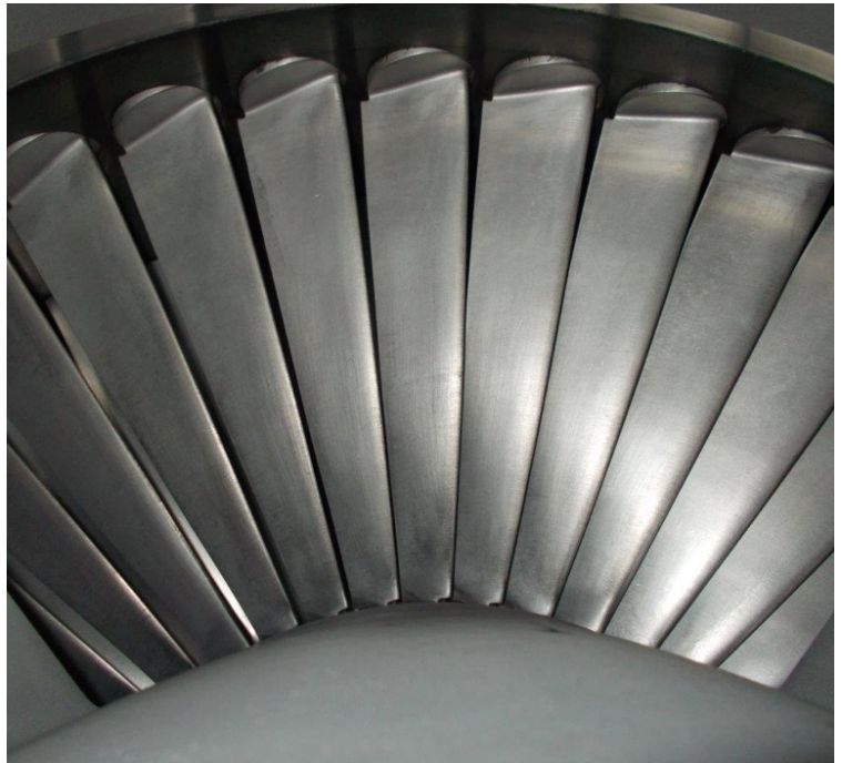
Clean blades after 4,000 hours with (H)EPA-grade Turbo-Tek Er5 | W5 | P1 watertight filters
