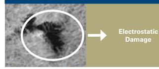
Donaldson Blue bulk fluid filters incorporates our best technology and construction to handle all fuels and lubricants in all operating environments. Donaldson Electrostatic Reduction Technology (D.E.R.T.TM) prevents filter media damage from electrostatic discharge. Epoxy is used in filter construction for increased fluid compatibility.
