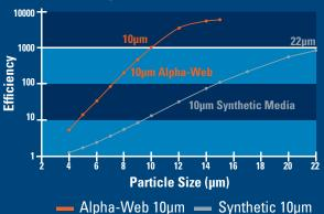
Donaldson's 10µm Alpha-Web media delivers better efficiencies in cyclic conditions compared to legacy 10µm synthetic medias. Alpha-Web offers higher efficiency with a lower restrictive pressure drop.
