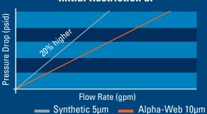
Donaldson's 10µm Alpha-Web and 5µm legacy synthetic medias are comparable in efficiency performance. The 10µm Alpha-Web allows for a 20% lower pressure drop than the legacy 5µm synthetic media. In mobile hydraulic applications where high efficiency is required but restriction is a concern, 10µm Alpha-Web provides a significant benefit to legacy 5µm media.
