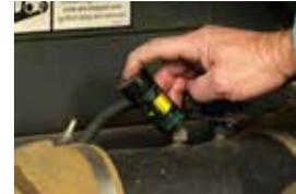
**2 Empty the Dust Cup & Check the Vacuator™ Valve**
