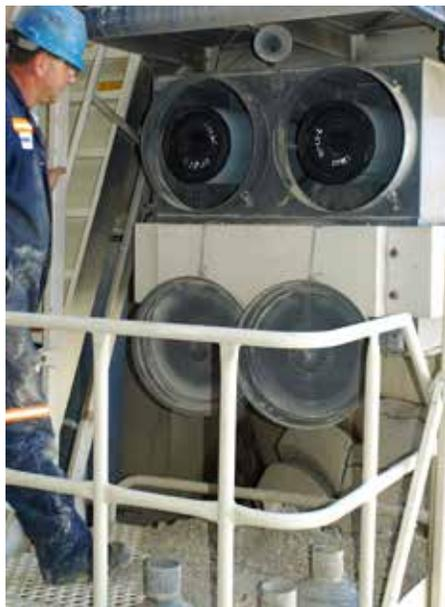
*Note: NEVER use the service cover to push the filter into place! Using the cover to push the filter in could cause damage to the housing or cover fasteners and will void the warranty.*
