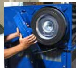
*Note: If you perform filter maintenance service on a schedule vs. using service indicators, you may want to write the service date on the filter end cap.*
