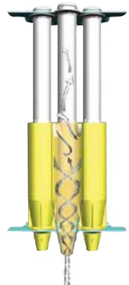
The pre-cleaned dust is automatically ejected from the dust cup with a Vacuator™ Valve, which is located below the lower housing body.
