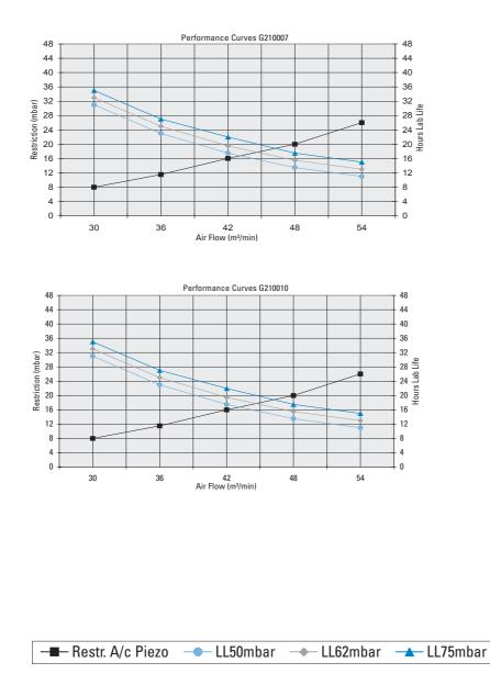
All performance curves are according ISO 5011 standards - Restriction measured at Piezo All tests are done with ISO Coarse at Dust Concentration of  $1g/m^3$
