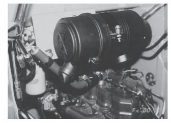
Despite its compact size, the FPG Air Cleaner offers complete engine air protection — removing 99.99+% of the dust and dirt particulate that enters the engine airstream.
