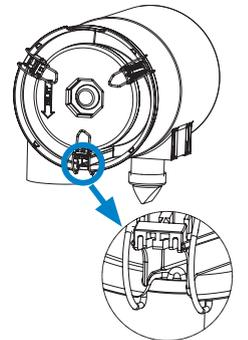
Refasten latches to secure cover. Make sure that latches penetrate the slots in both the body and the cover.
