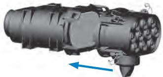
**7 Replace the service cover.** On PSD08, tilt the service cover into place and secure latches. For the PSD09, PSD10 and PSD12, place the service cover in position and fasten the latches. **Note:** If the cover doesn't seat, remove and re-check the filter position. The cover will be difficult to install if the filter isn't installed correctly.
