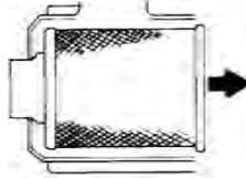
If your air cleaner has a safety filter, replace it every third primary filter change. Remove the safety filter as you would the primary filter. Make sure you cover the air cleaner outlet tube to avoid any unfiltered contaminant dropping into the engine.
