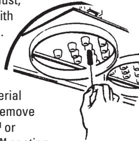
**Cleaning Note:** Never clean Donaclone™ tubes with compressed air unless both the primary and safety filters are installed in the air cleaner.
