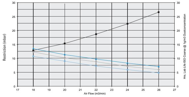
Performance Curves PSD120037/38 acc. ISO5011 with Vacuator Valve (vertically installed)
