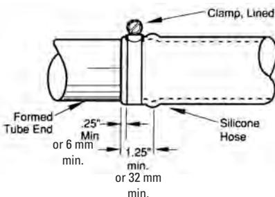
Initial torque on lined hose clamp should be 4.6 Nm. If retorquing is required, limit to 2.3 Nm.
