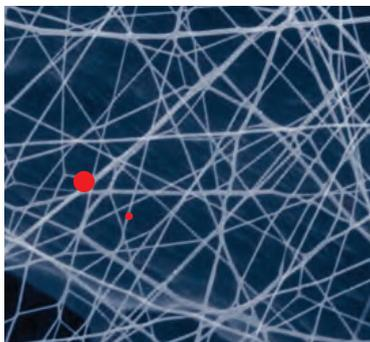
Ultra-Web fibers have submicron diameters and small interfiber spaces, which result in more contaminant being captured on the surface of the media and low restriction.
