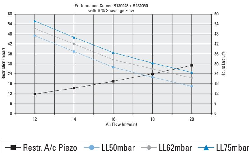
All performance curves are according ISO 5011 standards - Restriction measured at Piezo
