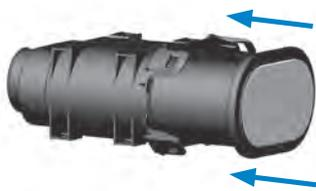
**6 Insert the primary filter.** For PSD08, slide the filter into the housing until the gasket seats against the housing. For PSD09, PSD10 and PSD12, slide the filter down at approximately a 5° angle until it hits the end of the housing. Rotate the filter toward the outlet section to complete the seal.
