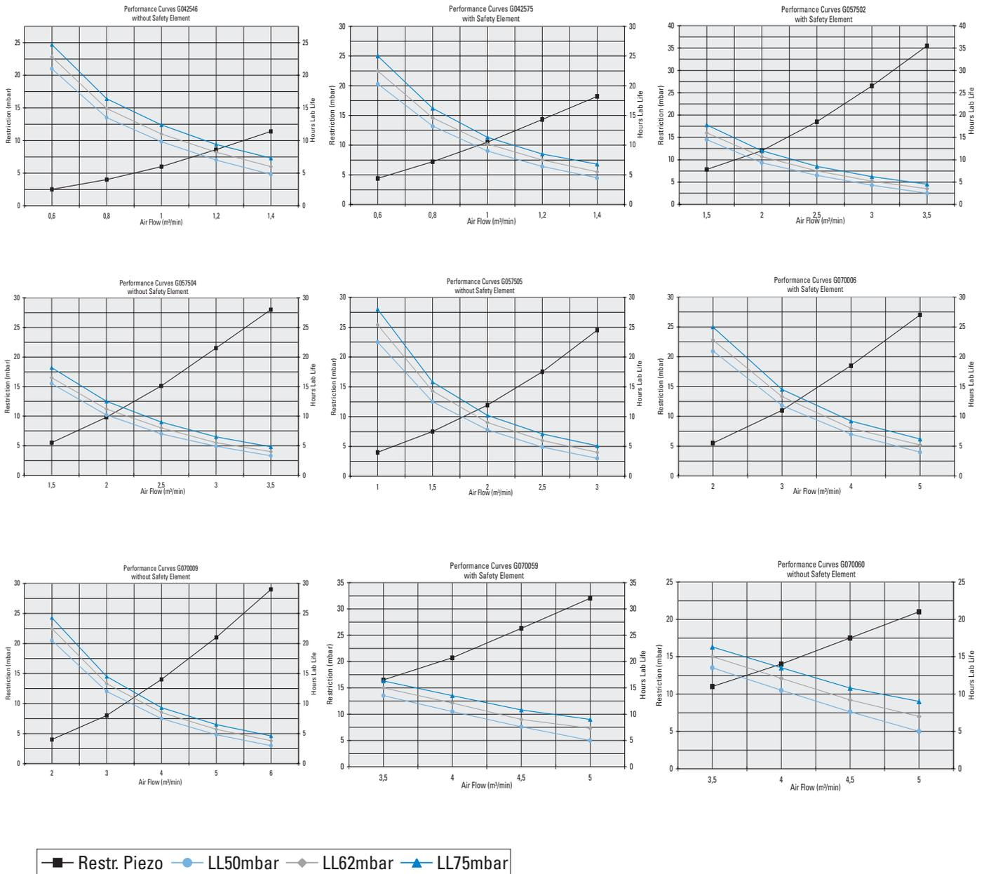
All performance curves are according ISO 5011 standards - Restriction measured at Piezo
