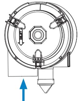
**APPLICATION NOTE** Never use the service cover to push the filter into place! Using the cover to push the filter could cause damage to the housing and will void the warranty.
