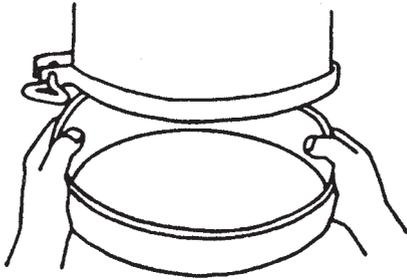
seals 360° around the air cleaner body. On dust cups with Vacuator™ Valve, dust cup service is minimal; just check the Vacuator™ Valve to see that it is not inverted, damaged or plugged. If it is damaged, replace it immediately.
