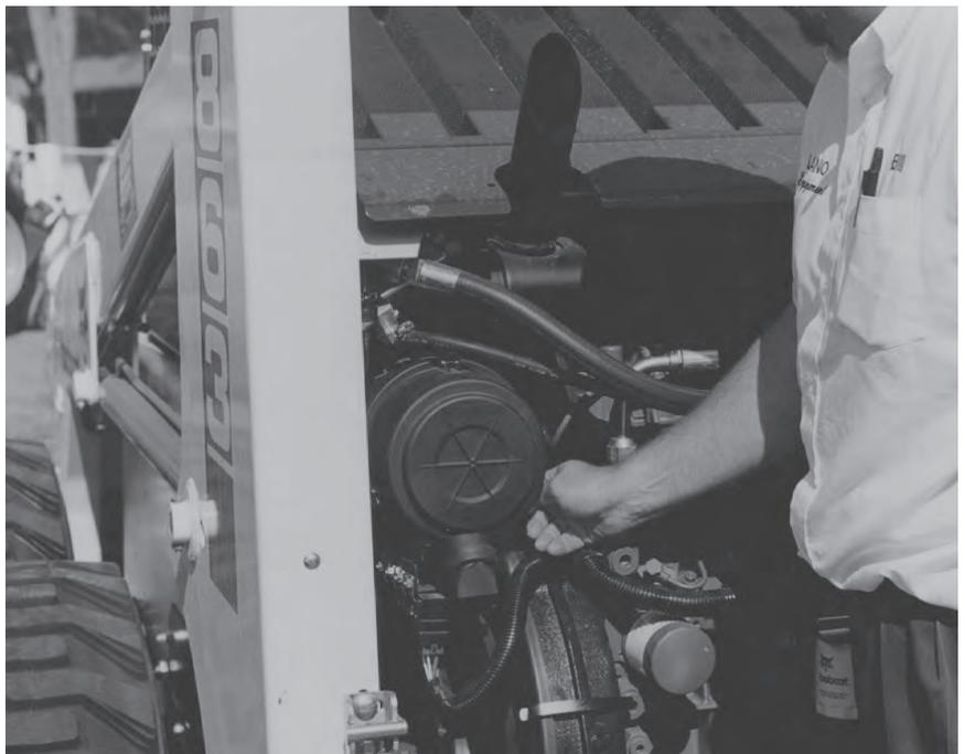
The filter inside the air cleaner is also quite different from the traditional design: one-piece molded urethane endcaps encase the ends of the media and filter liners, eliminating the metal caps and plastisol potting compound that were traditionally used. The glued-on gasket found on conventional filters is gone – now, the inside surface of the open end is actually the radial sealing surface.
