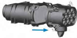
**1 Shut off engine. Unlatch and remove the housing service cover.**
