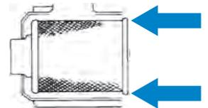
The critical sealing area will stretch slightly, adjust itself and distribute the sealing pressure evenly. To complete a tight seal, apply pressure by hand at the outer rim of the filter, not the flexible center. Avoid pushing on the center of the urethane end cap. No cover pressure is required to hold the seal. NEVER use the service cover to push the filter into place! Using the cover to push the filter in could cause damage to the housing, cover fasteners and will void the warranty.
