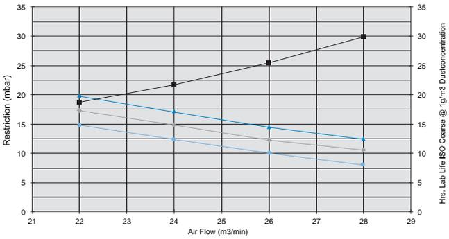
Performance Curves PSD120037/38 acc. ISO5011 with 10% scavange (vertically installed)
