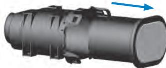
**2 Remove primary filter.** Pull the filter out of housing. On PSD09, PSD10, and PSD12 you must first loosen the filter gasket seal. Using the handle, push down on the filter to loosen the seal, which will tilt the filter to approximately a 5° angle.
