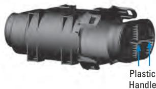
**3 Remove safety filter.** Using the plastic handle on the face of the safety filter, pull the filter toward the center of the housing and remove. **Note:** A safety filter only needs to be replaced at every third primary air filter change.
