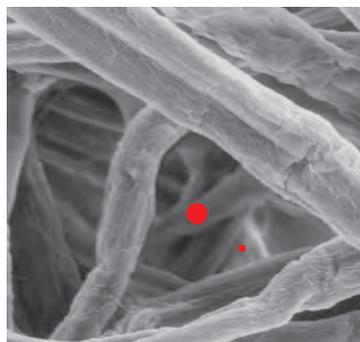
Cellulose fibers are larger than Ultra-Web fibers, and have larger spaces between the fibers, causing contaminant to load in the depth of the media and plug the airflow path; resulting in higher restriction and less capacity.
