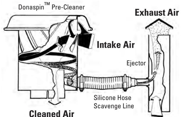
The Donaspin™ pre-cleaner uses a spinning motion of the airstream to force dirt and debris to the outside wall of the pre-cleaner body. The dirt and debris are forced to the bottom of the pre-cleaner and expelled by the secondary airflow developed by the ejector.
