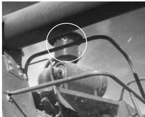
The Donaspin installed on this combine removes most of the incoming dirt, then directs the contaminant out of the system with the exhaust gases.
