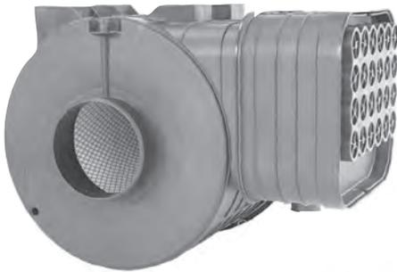
The SPB2 Air Cleaner is a two-stage full plastic air cleaner with built-in high efficiency Pre-Cleaner and RadialSeal™ Sealing Technology. They are suitable for agricultural and construction equipment operating in severe dust environments. To be used with an exhaust ejector. For all available Donaldson Exhaust Ejectors, see page 124-125.
