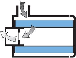
Air Cleaners in which the air goes through the inlet and directly to the main element are considered one-stage air cleaners. One-stage air cleaners are typically used where there is less contaminate in the environment, such as in on-road applications.
