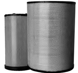
The critical sealing area will compress slightly, adjust itself and distribute the sealing pressure evenly. To complete a tight seal, apply pressure by hand at the outer rim of the filter, not the flexible center. (Avoid pushing on the center of the end cap.) No cover pressure is required to hold the seal. NEVER use the service cover to push the filter into place! Using the cover to push the filter in could cause damage to the housing or cover fasteners and will void the warranty.
