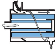
Air entering a two-stage air cleaner is first pre-cleaned before reaching the main element. The air may either be sent through pre-cleaner tubes or cleaned by centrifugal flow around the filter. Depending on the type of pre-cleaner, the pre-cleaner removes between 75-98% of the contaminate from the air before the air reaches the main element. Two stage air cleaners are recommended for use in medium- and heavy dust environments, such as in agricultural, construction, and mining applications.
