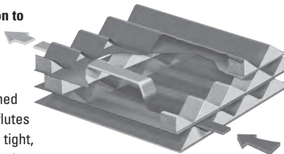
Filter media is formed into flutes - these flutes are layered to give tight, rugged structure to the filter
