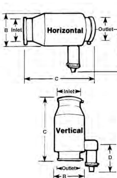
Horizontal model, for airflow of 3 to 40 m<sup>3</sup>/min.
