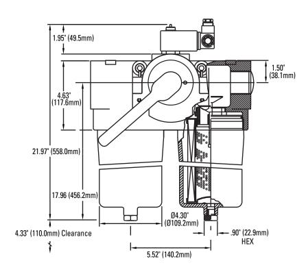
The handle shifts fluid flow from one filter to the other.
