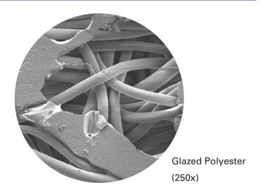
Needled 16 oz. glazed polyester felt is a versatile filtration media used in pulse jet baghouse dust collectors. The glazing process provides a better dust cake release by melting the outermost fibers and smearing them to create a smooth, high sheen surface. This material is strong, abrasion and chemical resistant and good for applications up to 275° F.
