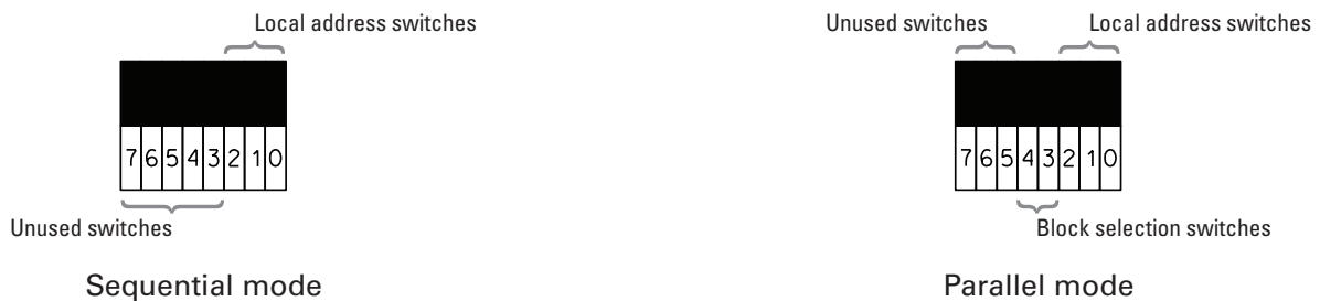
Figure 4: Configuration of the DIP switches on the STi Plus timer extension card
