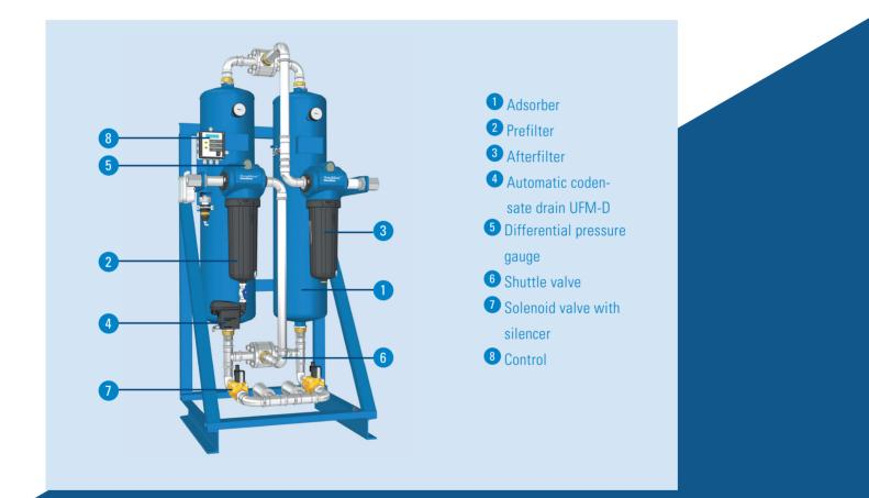
Adsorption dryers are always applied where highly purified and dry compressed air is required in accordance with ISO 8573-1.
