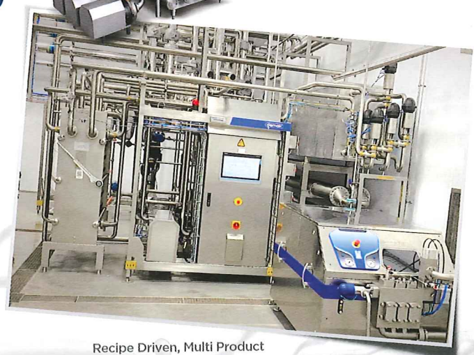
Space Saving CIP Module, 3 Channel, 5 Tanks
