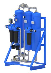
The Ultrapure HL- ALG dryer range is designed for drying and purifying of compressed air used in breathing or medical air applications reaching pressures up to 16 bar. The drying process is based on adsorption of water molecules out of a gas stream using hygroscopic desiccant materials. With this drying concept pressure dewpoints of -40°C (at 7 bar) or lower can be achieved. The unit also contains adsorbent that helps to remove other gaseous contaminates such as  $CO_2$ ,  $SO_2$  and  $NO_x$ .
